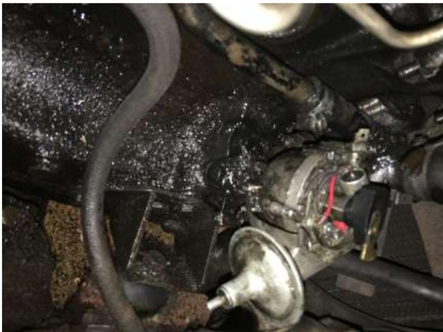
you actually want to work on. Trying to get round things in that engine bay is a bit like trying to peel a wet potato through a letterbox with sharp edges. So off came the bonnet, the air cleaner assembly, the battery and the carburettors. All of this takes about 30 minutes and the access and visibility gains reward that effort many times over. Now that I could see more, another
